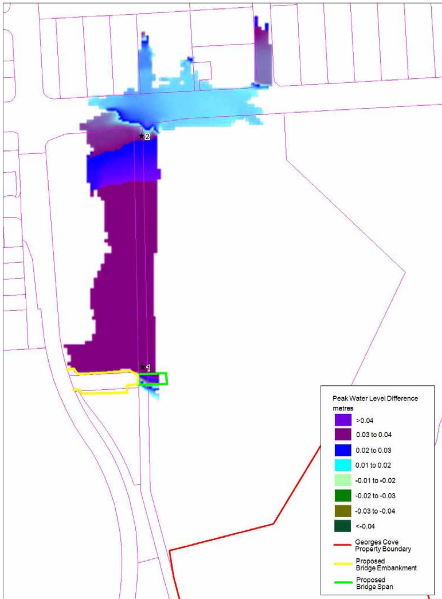
Figure 6 100 year ARI Local Flooding Peak Water Level Differences Post-Development - Road Bridge
